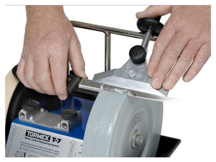
The SVM140 jig is made especially for long and thin knives. It works in the same way as the SVM45 jig but it is wider and therefore gives more support to long and thin blades.
