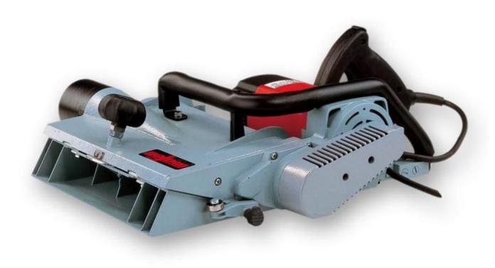
The Mafell ZH 320Ec is considered by most timber framers to be the finest wide format planer in the world. This 32cm planer is very lightweight at only 14kg, and extremely powerful. It has excellent sliding properties, even with moist timbers, due to special base-plate structure, and it even offers a new enhanced air duct for excellent chip removal.
