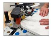
Edgebanding of straight, shaped, or beveled panels (up to 45°)
