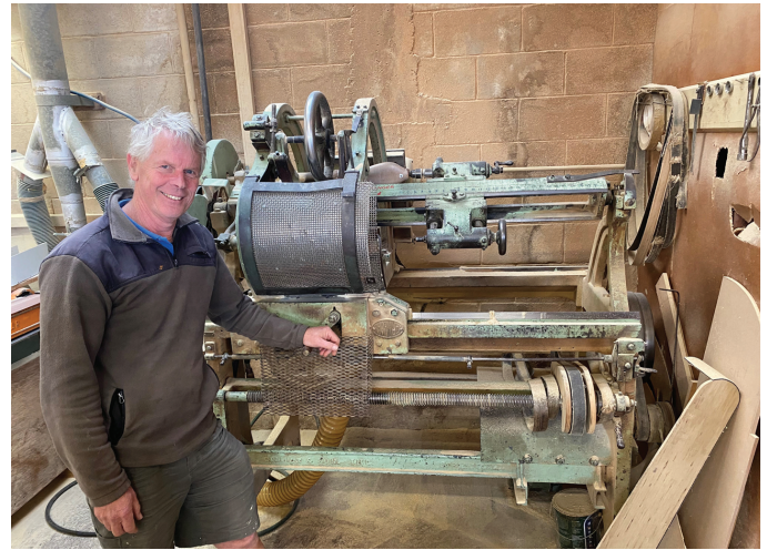
Peter in front of the copy lathe - made in the 1800's and still in use.
