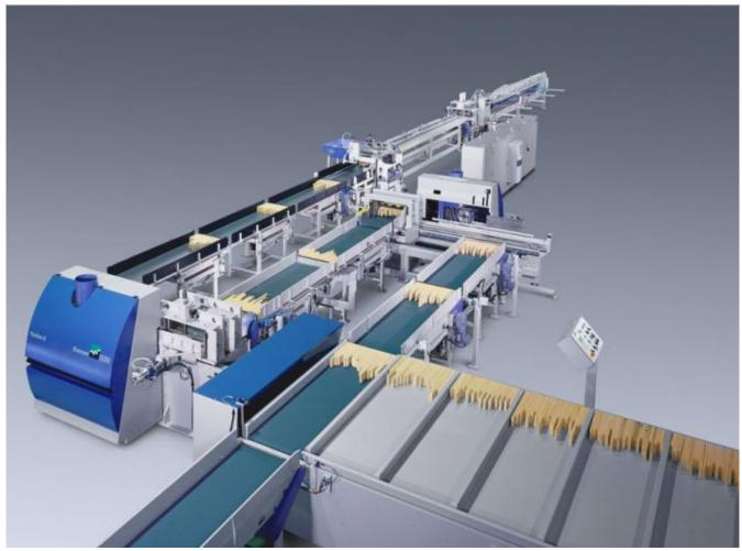
The Turbo-S finger jointing line is a Grecon-patented shaper combination for the production of horizontal and vertical finger joints that is characterised by its high capacity.
