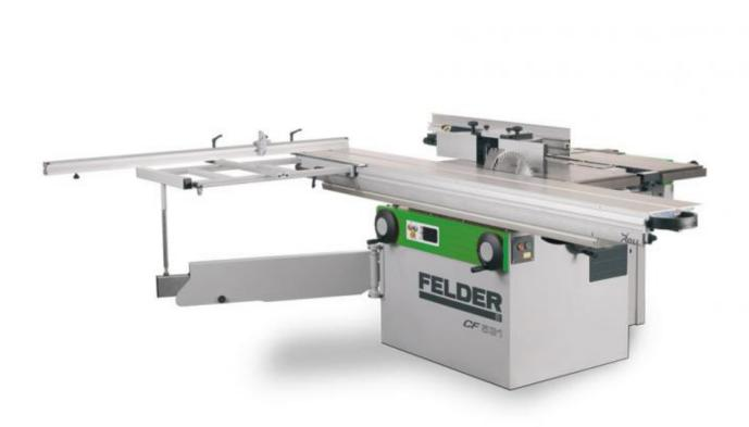
The CF 531 Professional is a true all-rounder of wood-working. Top quality planing, thicknessing, moulding, cutting as well as an option for mortising - all in such a small area.
